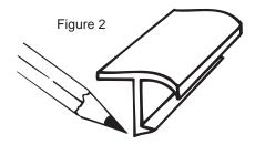
template accurately onto the countertop. 7. Measure across the metal mounting frame from side to side to locate its center. Mark this on the front of the frame. Move the frame to the desired position and mark the location of the centerline on the countertop. Measure the distance from the centerline to the nearest side wall or the end of the counter. Then measure the same distance from the side wall to locate the centerline at the back of the counter.
